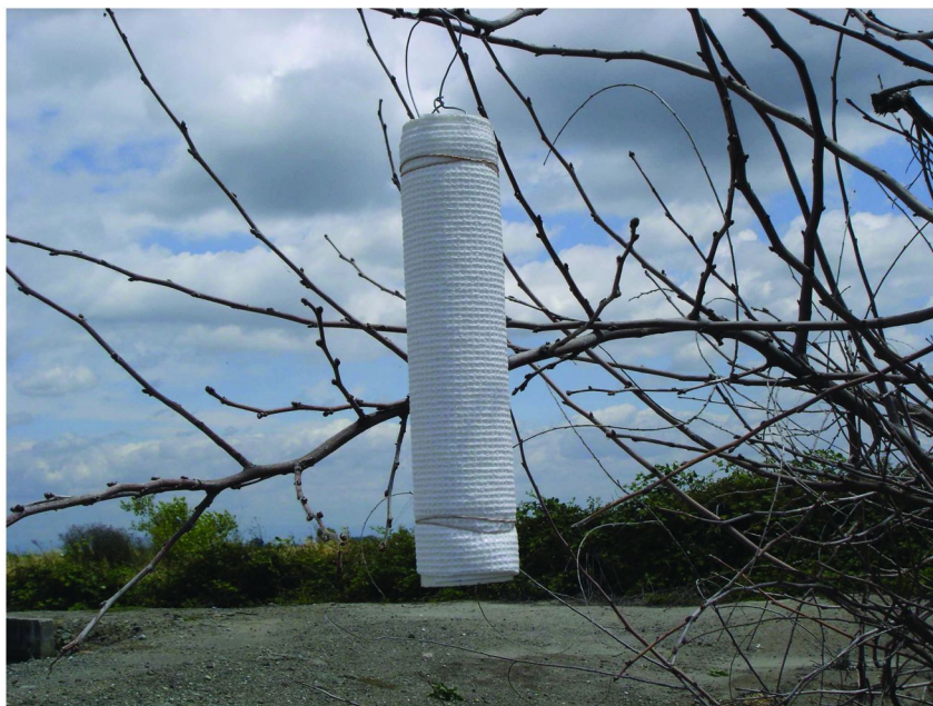
Figure 3. Sampling Sheet (Kimbie) Wrapped Around PVC Pipe and Suspended in Tree
